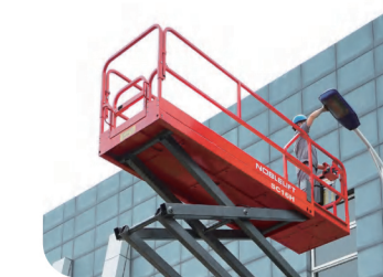
Extension platform Enlarged operating area and the ability to work over obstacles.
