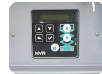
Fault code display Easier trouble shooting and maintenance. Automatically record operating time. User can perform periodic maintenance at the proper intervals.
